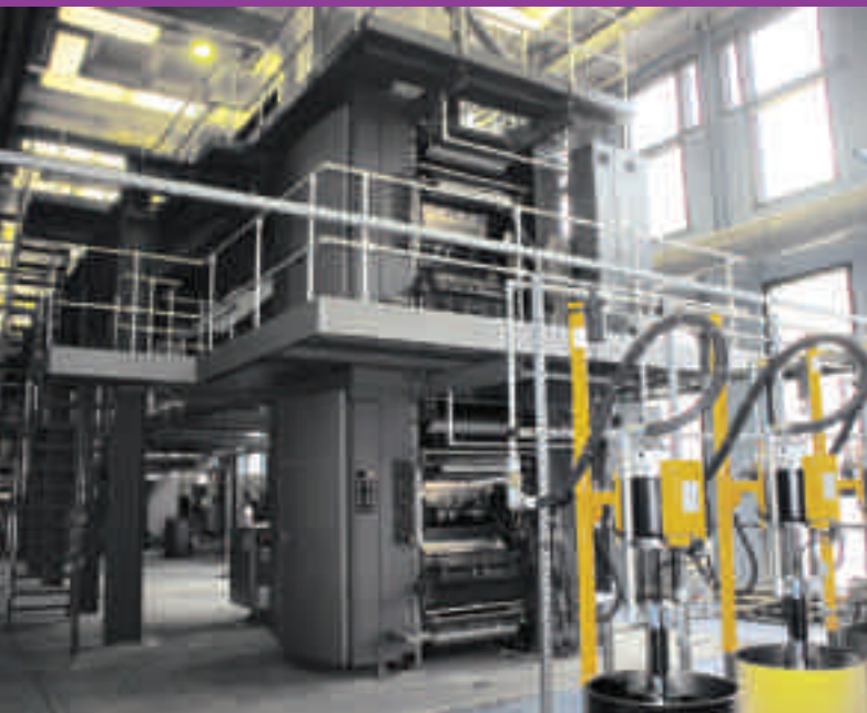
Two Goss Uniliner towers dominate the new 100% color capabilities at MNPP in Moscow.
